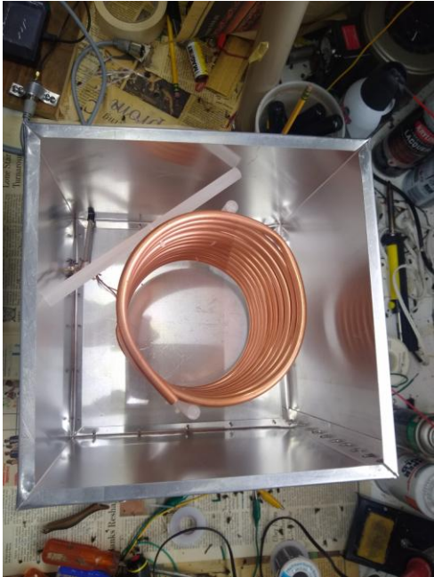
Figure 6 - A Coil Mounted in a Chamber on Rexolite Rods
