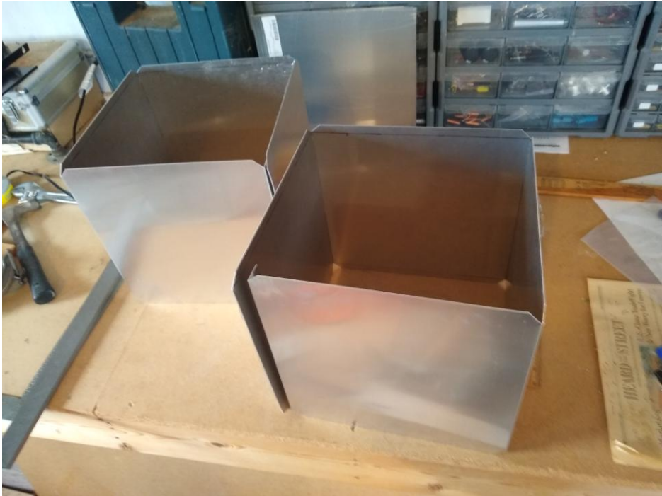
Figure 1 - Bending the Chamber Sides with the Brake
