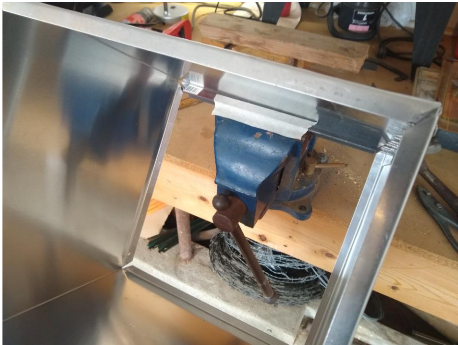
Figure 3 - Bending the Chamber Flanges to 45 Degrees on the Brake
