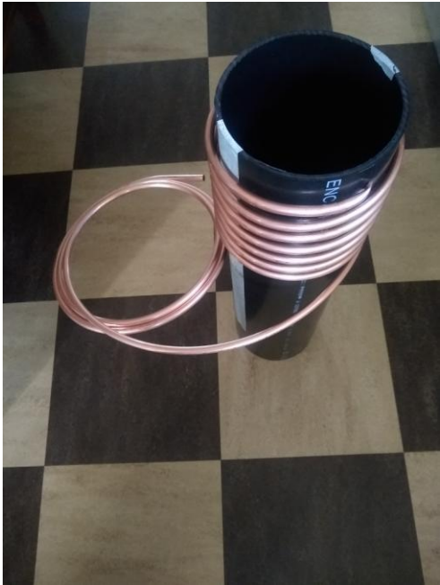
Figure 5 - Winding the 6.5 inch Diameter Coils
