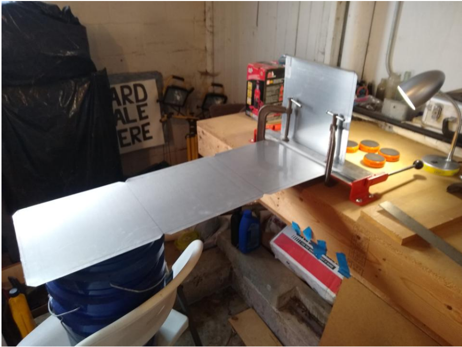
Figure 1 - Bending the Chamber Sides with the Brake
