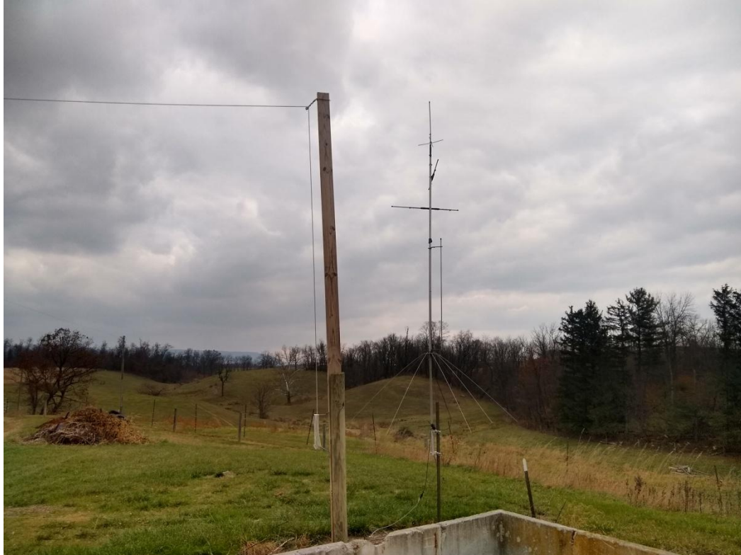
Picture 2: The transmit antenna was a multiband Cushcraft MA-5 operating on 20 meters
