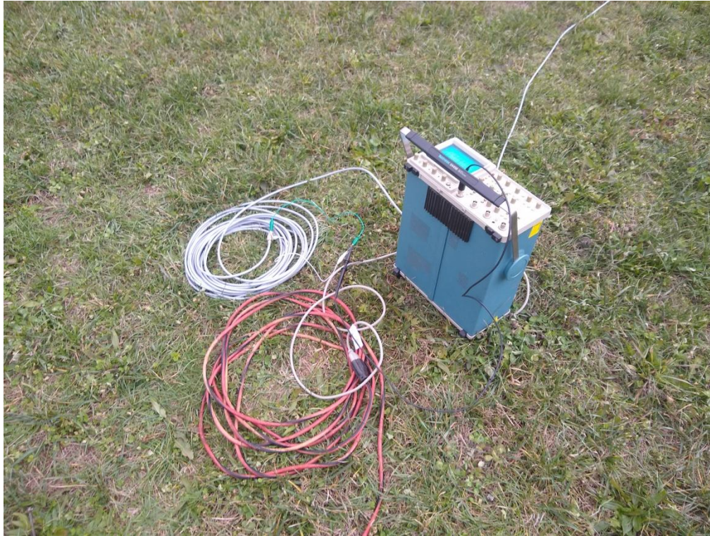
Picture 4: The signal on the receive or victim antenna was measured with an analog scope across a 50 ohm load
